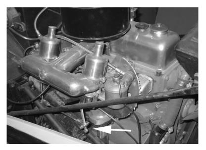
Heat shield with carburettors and linkage in place
