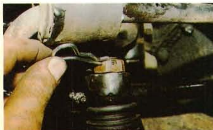
Castellated nuts never work loose, until the day you forget the split pin or R-clip.
