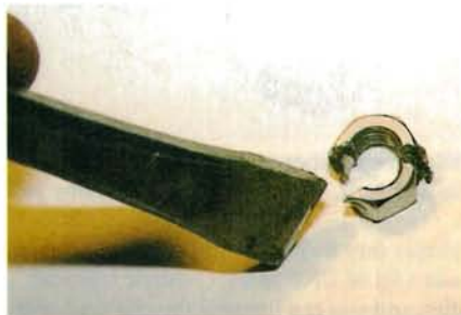
Sharp, cold chisel completes the job on the weakened nut without damaging stud.
