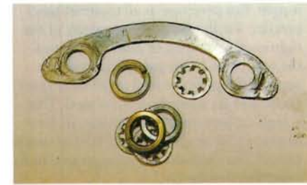
Shake-proof, spring and tab washers are all used with flat washers to eliminate fret.
