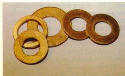
Copper washers are for sealing fluid joints. Collapsible ones are for single-use only.
