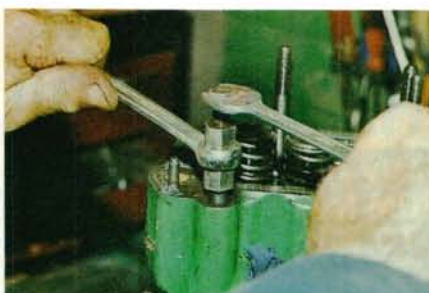
Home-made tool gets stud out undamaged, but you'll need a centre lathe to make it.
