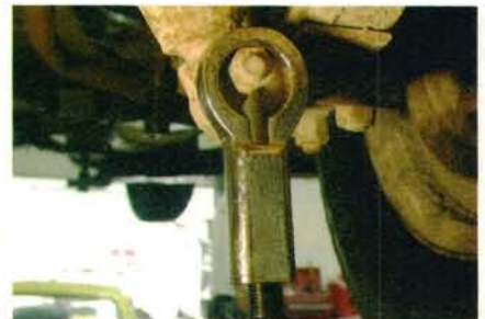
Nut splitter is effective and inexpensive, but requires plenty of room for access.
