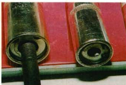
Commercial stud removal tools are also effective, but they can damage threads.
