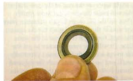
Doughty washer is flat metal with a rubber seal in the centre. It also holds fluid in.
