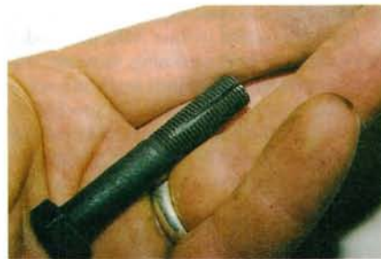
Home-made tap can be very effective at cleaning minor damage to female thread.
