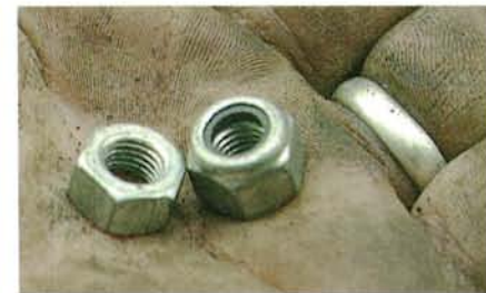
Nyloc nut has rounded top to contain a nylon insert. They can only be used once.
