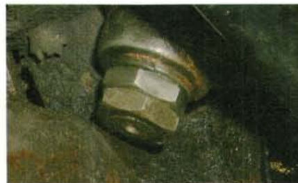
Two half nuts or 'jamming nuts' wound tightly together can act as effective lock.
