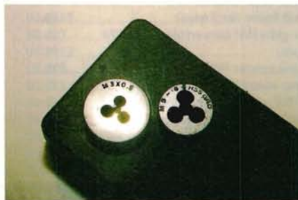
Solid die (left) can't be adjusted for fine changes, unlike the split one (right).
