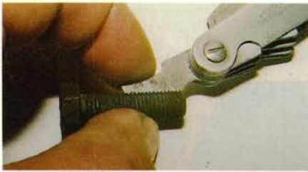
Use a thread pitch gauge to accurately measure how many teeth there are per inch.
