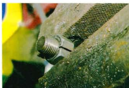
Sacrifice a nut, and you can hold studs or bolts in a vice without fear of damage.
