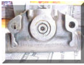
Figure 1: This is what lurks behind the disk and disk gasket. After disk was removed, the damper was placed with this side up and the entire disk area was filled with penetrating oil. I let it soak for several days, keeping this area full. Idea is to make pressing the shaft out as easy as possible. Don't forget to place folded paper towels or rags on the under side to catch oil once it penetrates through.
