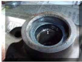
Figure 3: First seal in place. Ensure hole (arrow) is clear of obstruction (see text). Second seal fits in place right on top of this one.
