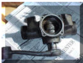
Figure 2: Center punch marks (highlighted here with white paint) on piston crank (top mark) and body. Similar marks made on outside body and arm. After seal installation, marks are used to align shaft, arm and piston crank, so that all will be in the same relative position as when removed. (Note that picture shows shaft after it has been pressed out, hence the gap between the body and the arm).
