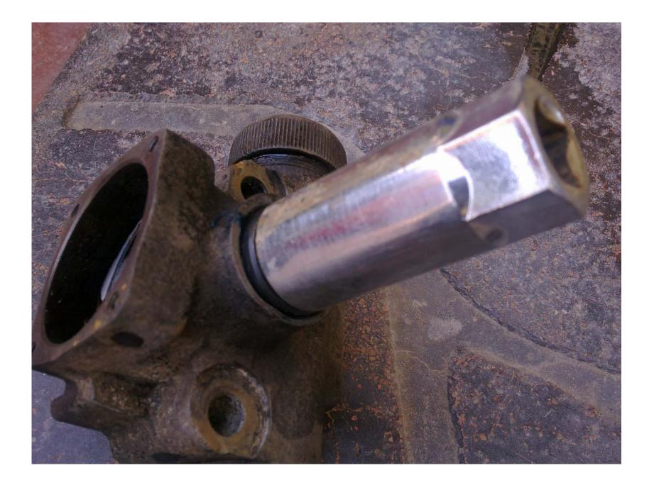
To get the seal in nice an d tight, use a non sharp object to push the seal in further. Be careful not to push too hard. Tap slightly on all four sides, allowing the seal to equally slide in.
