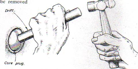
Figs. 3 and 4.—(Left) The core plug seating must be carefully cleaned of rust, etc., and a little gasket cement evenly applied. (Above) The new core plug is reinstated by applying a drift and gently tapping with a hammer. It should be noted that the plug is not flattened, but still retains most of its convex shape.
