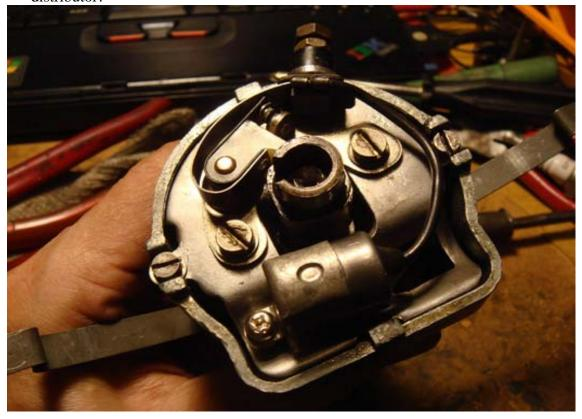
8. Depending on the manufacturer of the condenser you choose the exact wiring may be slightly different from the one shown above.
