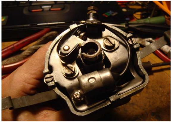
9. Here is yet another different manufacturer's condenser. Note the position of the hold down screw has moved. Just drill a new hole and tap it to fit the new hole location on the condenser.
