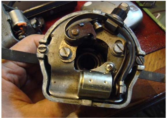
10. What condenser should I use on my DKY4A distributor in my MG Y? The MG MGB condenser is a very suitable and compatible condenser to fit instead of the original.
