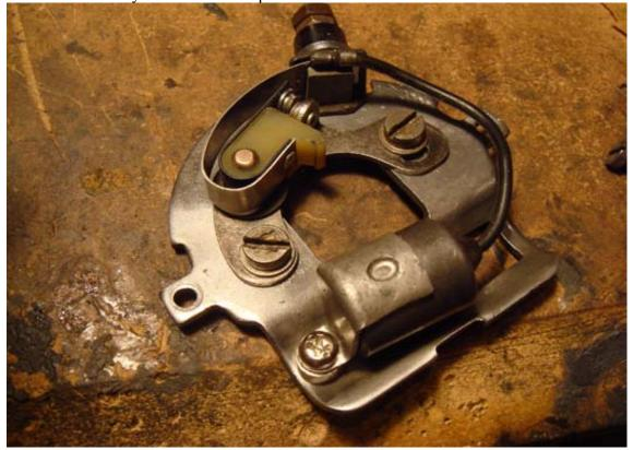
7. Refit the base plate to the distributor and you can gap and set the points before refitting the distributor to the car. This is the easy way to set up the distributor!
