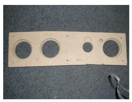
The veneer is cut with enough overlap all round the holes to allow an octagonal hole round which the trim pushes on the veneer only. The trim was cut with a sharp knife to fit the octagon shape and no adhesive is needed as long as the joints are tight.
