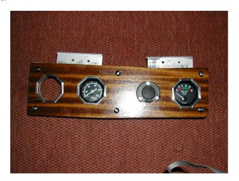
The panel was fixed to the back of the dashboard with two aluminium strips, bolted to the panel before assembly. I thought that I screwed these but looking at the pictures, it is clear that I bolted it with bronze mushroom headed machine screws which will also have come from my everlasting stock of junk saved over the last fifty years.
