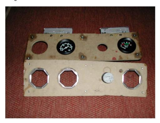
I chose to join the panels together using large headed chrome machine screws in to captive nuts in the rear panel fixed with epoxy glue, but this was largely because I already had these. I'm sure that a method of secret fixing could be devised.
